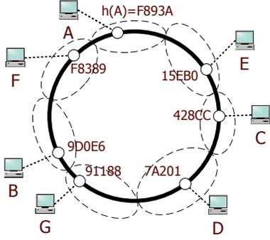
**Figure 1. An example ID space for a structured overlay, represented as a ring. The nodes maintaining the overlay are represented as white circles on the ring; for example, computer A is represented as the circle with ID  $h(A) = F893A$ . Dashed ovals represent the “responsibility” of every node, in terms of the ID range it manages. In this example, every node manages the range of IDs that are numerically closest to its own identifier.**
