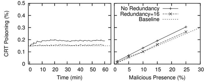
**Figure 5. ConsRT poisoning without redundant routing and with 16-path redundancy. (a) Time graph of ConsRT poisoning for 15% malicious presence. (b) Steady-state ConsRT poisoning for different malicious presence levels.**
