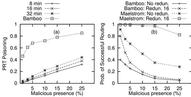
**Figure 7. OptRT security characteristics vs. malicious presence in the population. (a) Routing-table poisoning for different Maelstrom epoch lengths and for Bamboo. (b) Probability of successful lookup delivery for different redundancy levels for Bamboo and Maelstrom.**
