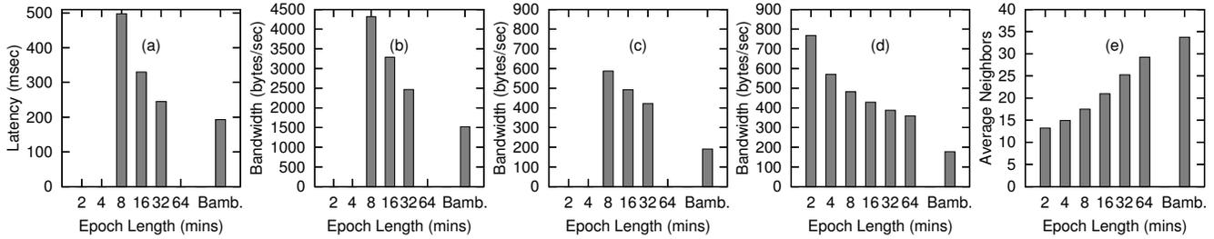
**Figure 8. Performance measurements as a function of epoch length, compared to Bamboo. (a) Lookup latency from algorithmic simulator (50,000 nodes); (b) & (c) Maintenance bandwidth from the algorithmic simulator, 50,000 and 500 nodes respectively; (d) Maintenance bandwidth from the implementation (500 nodes); and (e) Average number of neighbors per node from the implementation (500 nodes).**
